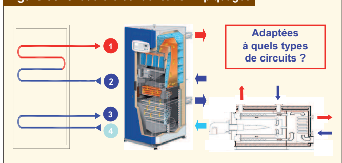
Figure 5c. Chaudière condensation 4 piquages
